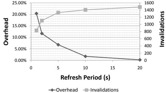
Figure 5: Overhead and Invalidations vs. Refresh Period. Apache Build on Linux. Averages of five runs with standard deviations below 2% of the average.
