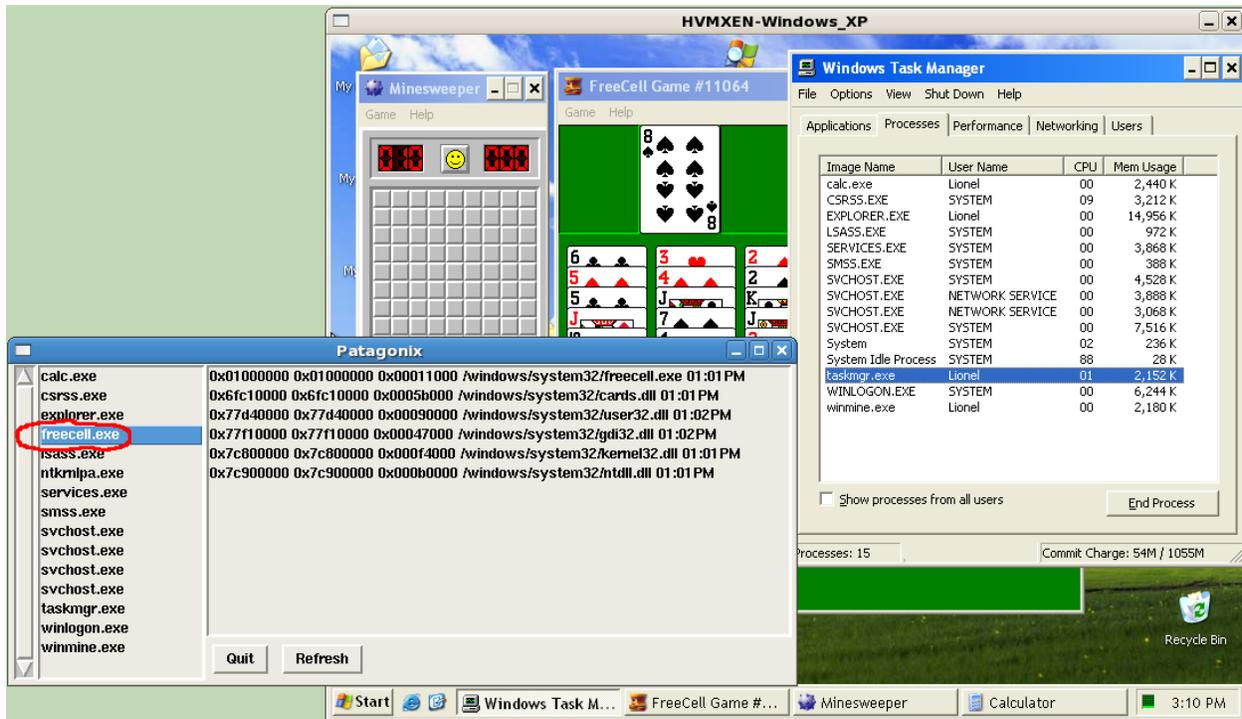
Figure 3: Output of both Patagonix and the Task Manager when the FU rootkit is used to hide `freecell.exe`. Patagonix identifies all processes including `freecell.exe`, while the Task Manager does not display the hidden process. Patagonix identifies “System” as `ntkrnlpa.exe`, the name of the Windows XP kernel binary.
